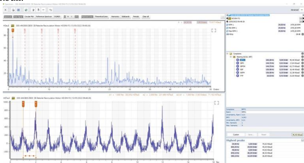
Gambar 10. Spectrum DE Reboiler Recirculation Motor Before Repair
