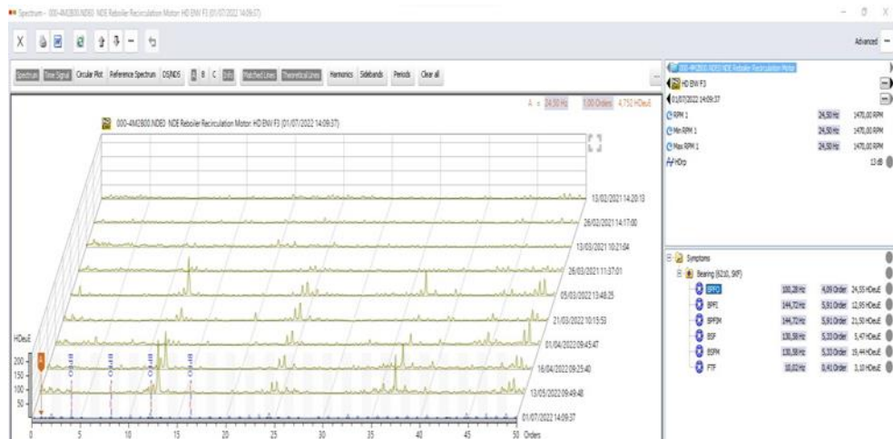
Gambar 9. Waterfall NDE Reboiler Recirculation Motor
